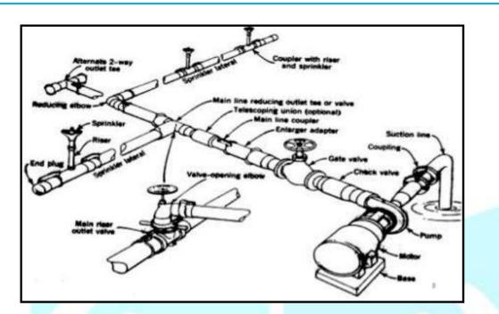
The following tabular column shows various parts of a sprinkler system
